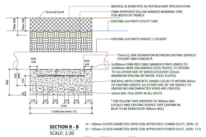
Figure 11 - Example of 110kV UGC Cable Undercrossing
