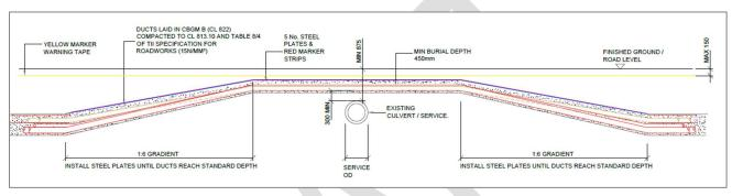
Figure 13 - 110kV UGC Culvert Overcrossing
