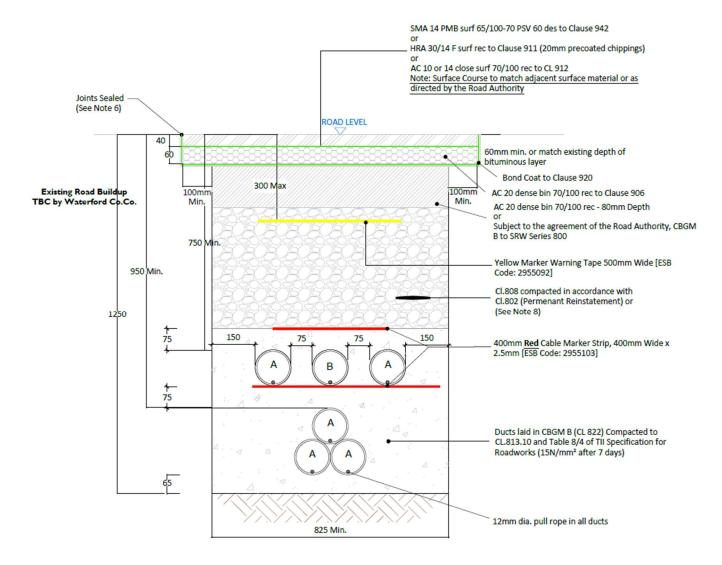
A = 125mm: Outer Diameter HDPE ESB Approved Duct, SDR=17.6 (Power) [ESB Code: 9317552]
