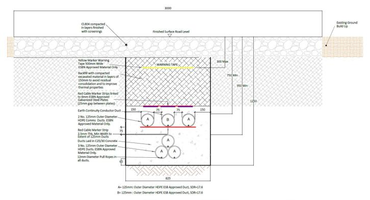
Figure 5 - Trench in Off Road Section
