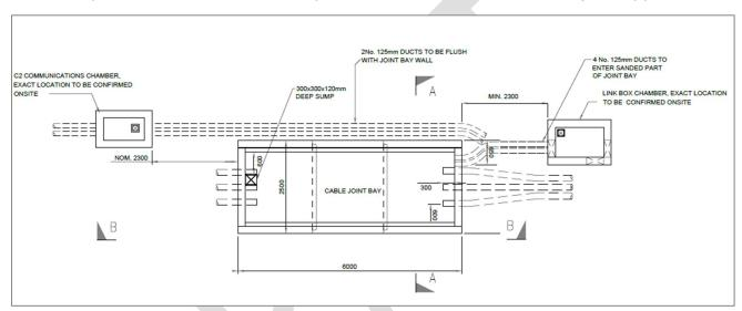
Figure 7 -110kV Joint Bay Plan Layout
