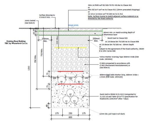
A = 125mm: Outer Diameter HDPE ESB Approved Duct, SDR=17.6 (Power) [ESB Code: 9317552]
