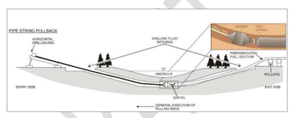
Figure 20 - Example of HDD Installation
