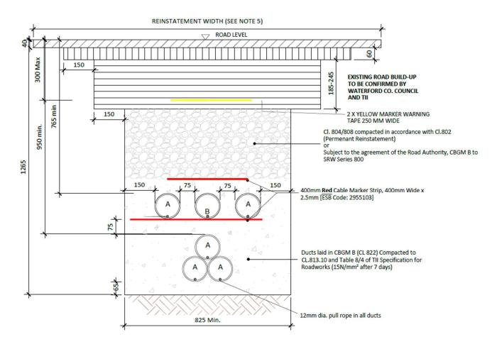
A = 125mm: Outer Diameter HDPE Duct, SDR=17.6 (Power)
