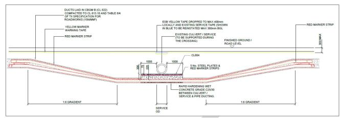
Figure 12 - 110kV UGC Culvert Undercrossing
